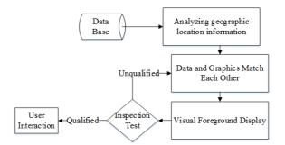
Fig. 2. Design flow of visualization module based on space
