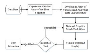
Fig. 6. Design flow of visualization module based on time sequence
